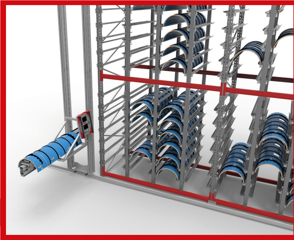
Rotary die storage system with stacker crane
